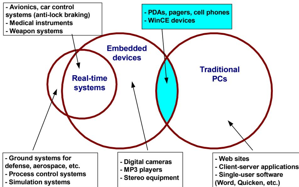
Figure 1: How embedded devices with fully featured operating systems relate to other devices
