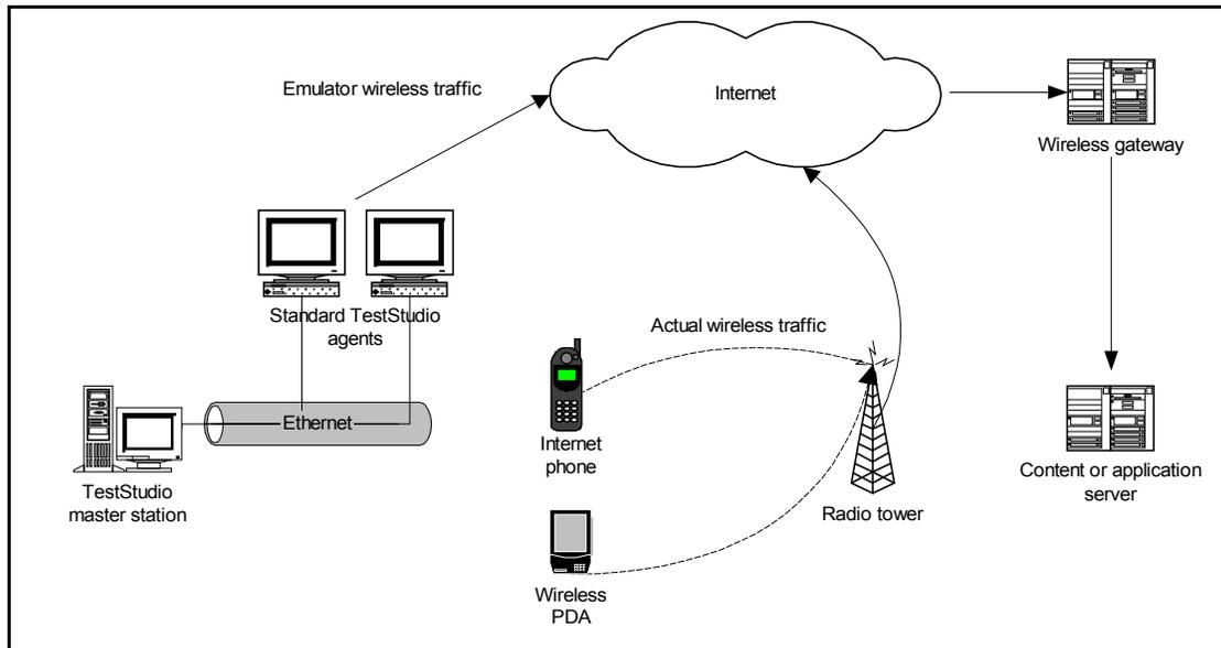
**Figure 3: Performance testing using an emulator that connects to the wireless gateway via the Internet**
